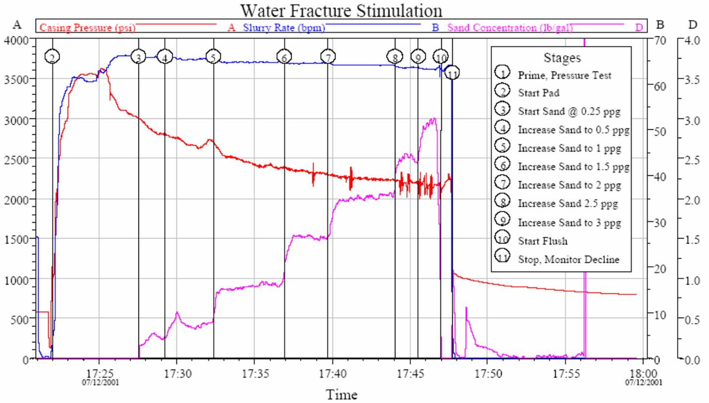
Figure 5 Well Number 30 Stage 1 Fracture stimulation of the DI and Du Seam
