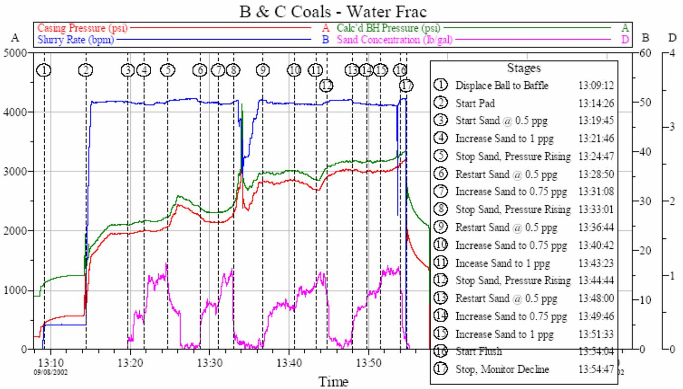
Figure 4 Well Number 19 Stage 2 Fracture stimulation of the B and C Seam
